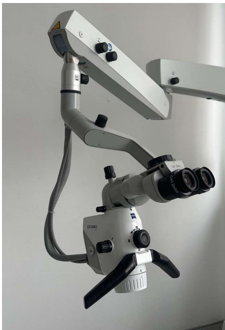
Fig. 2. Dental operating microscope (DOM) (Extaro 3000, Carl Zeiss Meditec, Germany) that was used in the study
